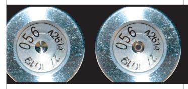
Unfit Control Value (at the right side) and control grinded Control Valve (at the left side)
